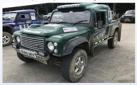
Alex started racing in 1998 with an original Bowler Tomcat. The current car was built in 2004 and it has a 4.8 V8 coupled to a standard four-speed Range Rover automatic gearbox.
